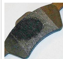
Friction material contaminated with oil. grease or brake fluid
