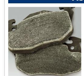
• Partially charred friction material (whitish outer edges)
